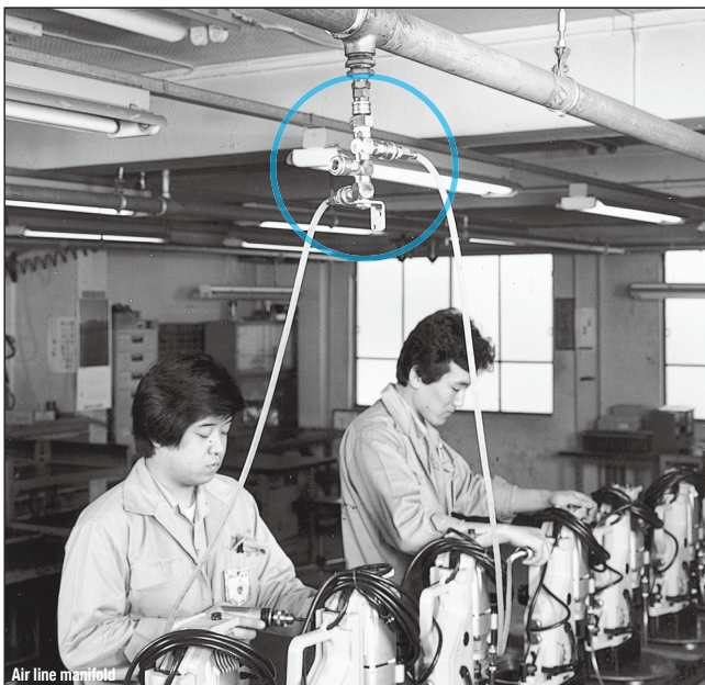
Air line manifold
